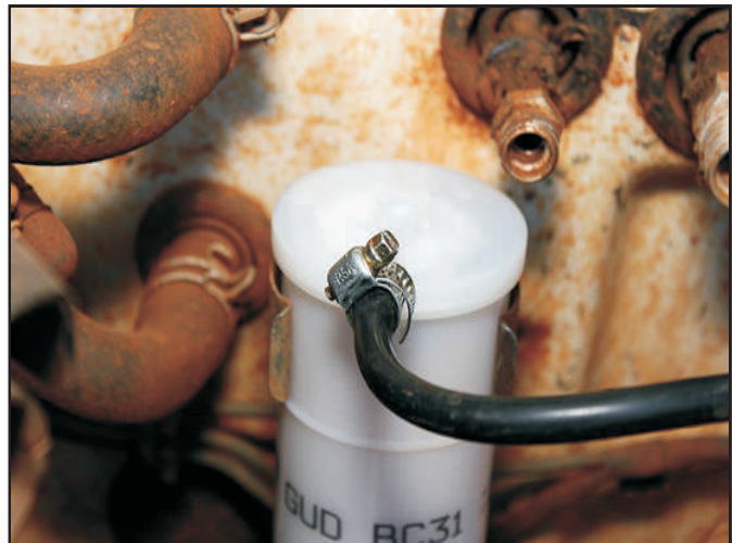
Fig.: Changing of Oil Filter
